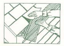
Repairs will need to be made to leaky gutters or, if not repairable, the section which leaks should be replaced. Downspouts should direct the water away from the foundation to prevent eroding the soil along side the house and to keep moisture from the crawl space or basement.
