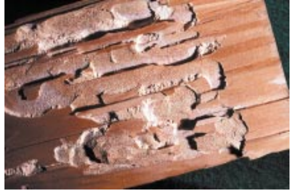
Fig. 5b. Buprestid beetle larval mines.
