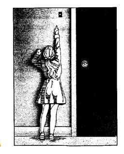
The pushbutton wall control should be out of reach of children (at least 5 feet from the floor) and away from all moving parts. Mount and use the button where you can clearly see the moving garage door.
