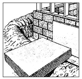
**RIGID INSULATION** is made from fibrous materials or plastic
