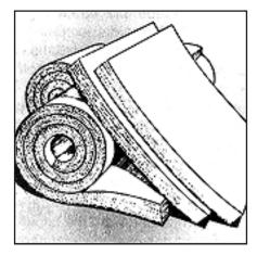
**BLANKETS,** in the form of batts or rolls, are flexible products made from mineral fibers. They are available in widths suited to standard spacings of wall studs and attic or floor joists. Continuous rolls can be hand-cut and trimmed to fit. They are available with or without vapor retarder facings. Batts with a special flame-resistant facing are available in various widths for basement walls where the insulation will be left exposed.
