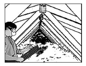
**BLOWN-IN** loose-fill insulation includes loose fibers or fiber pellets that are blown into building cavities or attics using special pneumatic equipment. Another form includes fibers that are co-sprayed with an adhesive to make them resistant to settling. The blown-in material can provide additional resistance to air infiltration if the insulation is sufficiently dense.
